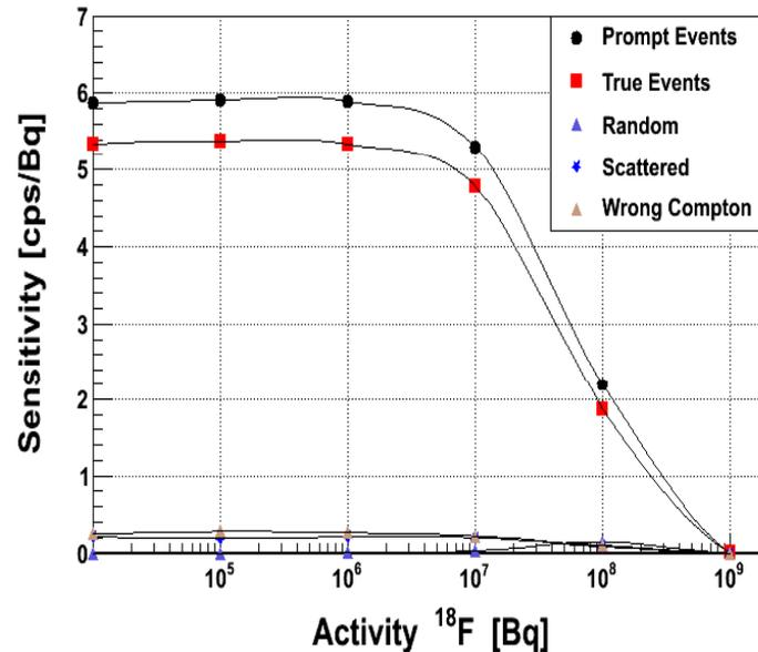
VIP Compton camera sensitivity for different activities of <sup>18</sup>F isotope. The good energy resolution of the CdTe detector allow us to discard most of the random and scattered events achieving a signal-to-noise ratio of 93%.
