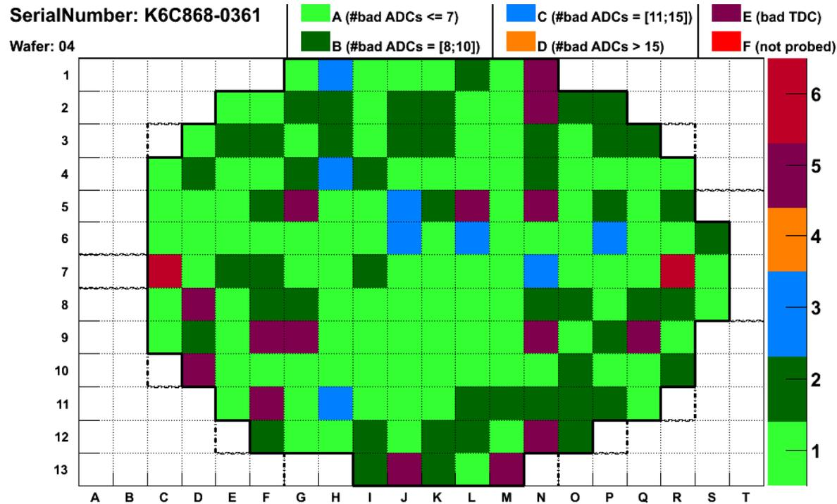
Typical results after probing. Each wafer can provide enough chips of class A for 2 Modules (80 chips)
