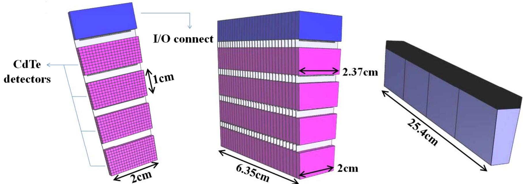
**VIP detector module** is made of pixelated CdTe detectors with trapezoidal shape. It is bonded to the thinned ROC and then
