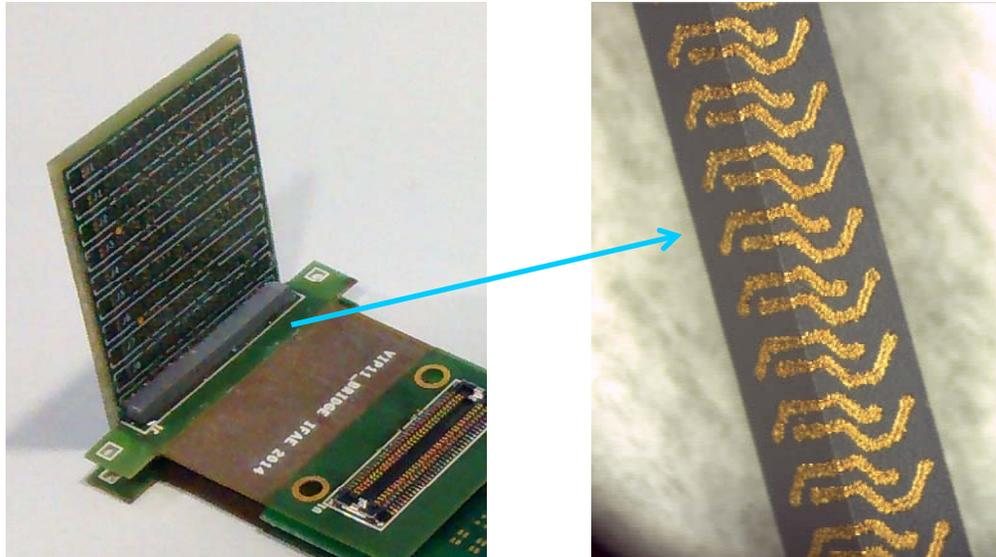
Original design was based on 3D plastic PCB but after long R&D we realized that it does not fit for 250um solder balls. We decided to go for 3D Ceramic PCB. The delivery will be by end of November
