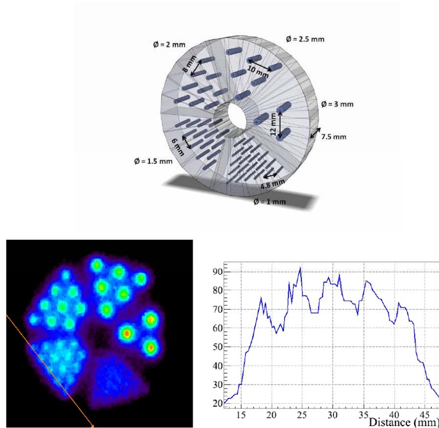
FIGURE 6.28: *Top*: scheme of the phantom. *Bottom*: reconstructed image with LM-OSEM and corresponding line profile of the 1.5 mm diameter rods. [75]
