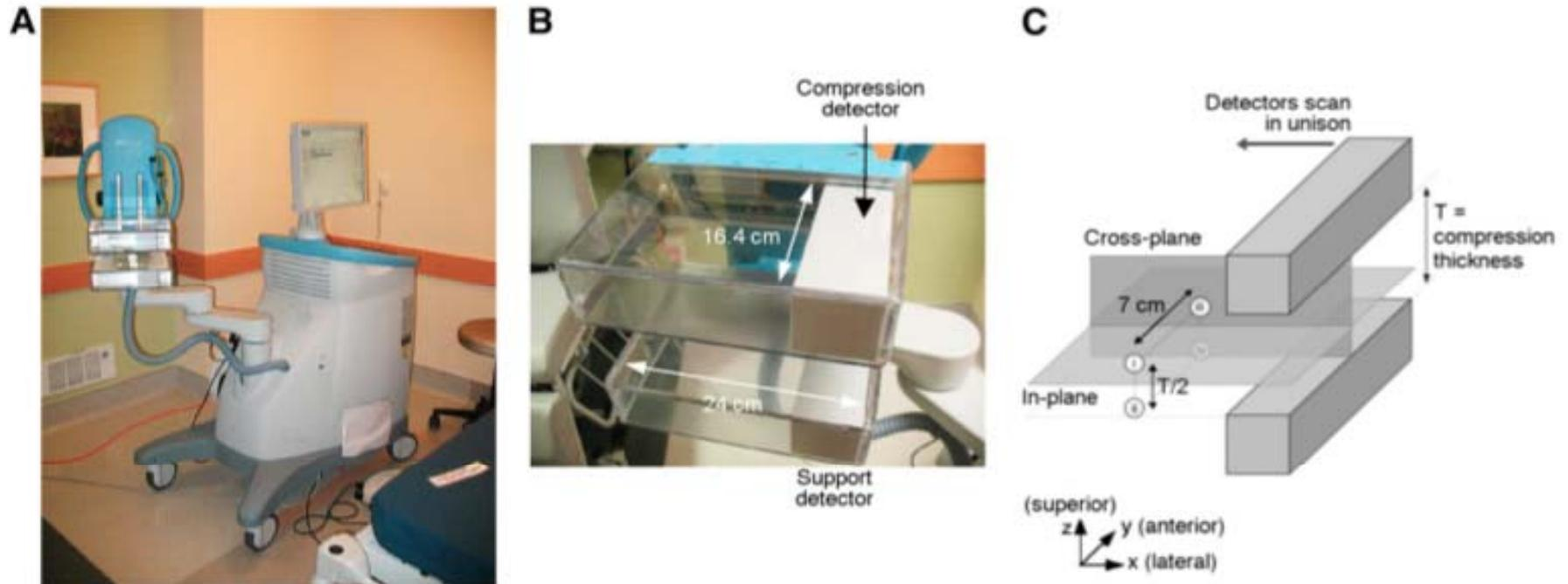
**FIGURE 1.** (A) PEM Flex Solo II system. (B) Close-up of detectors. (C) Illustration of in-planes and cross-planes. Four cardinal positions (i, ii, iii, and iv) within PEM Flex FOV used to investigate quantification consistency.
