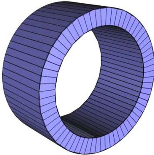
When 66 of the VIP sectors are put together, they form a cylindrical seamless PET scanner. A total number of the detector voxels is 6,336,000. Thus, the VIP has 6,336,000 independent readout electronic channels.
