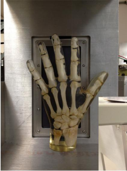
Hand Phantom imaged with 200 MeV protons at the Loma Linda Synchrotron, using the existing pCT scanner.
