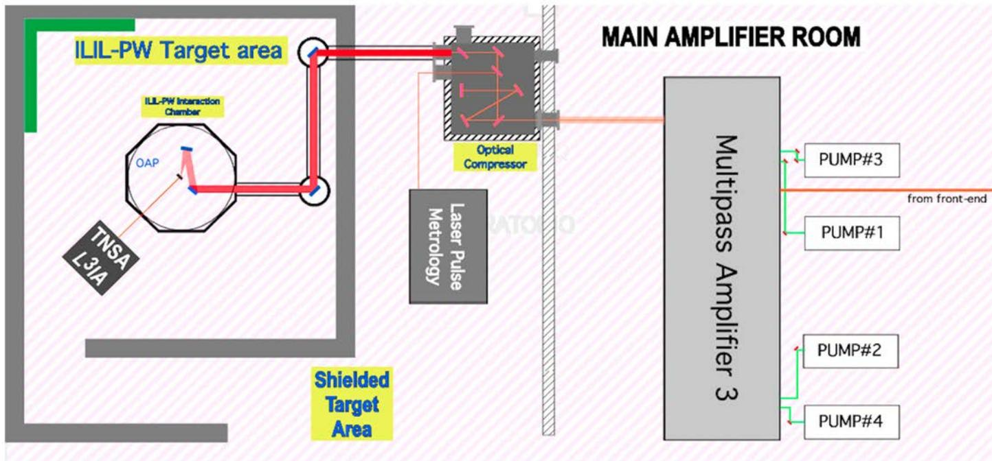
Figure 1: Lay-out of ILIL-PW system comprising the main multi-pass amplifier, compressor, and target area [2].
