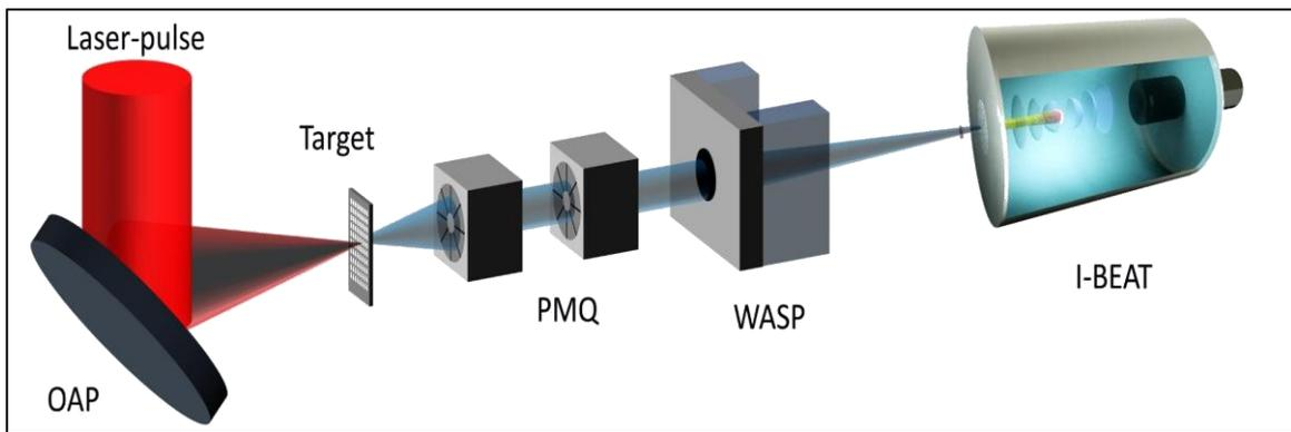
Figure 1: Schematic drawing of the I-BEAT integrated in a beamline for laser accelerated ions. The laser pulse is focused via an off-axis parabolic mirror (OAP) onto a target, from which the ions are accelerated. Two permanent magnet (PMQ) are installed to focus the ions and a wide angle spectrometer (WASP) filters out electrons and low energy particles. The ionoacoustic signal of the particles in the I-BEAT detector is recorded with a transducer (visible in black).
