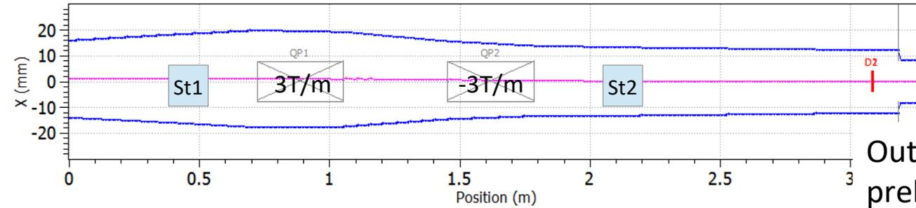
Out of PMQs+ESS used in input for preliminary simulation of last beam-line section
