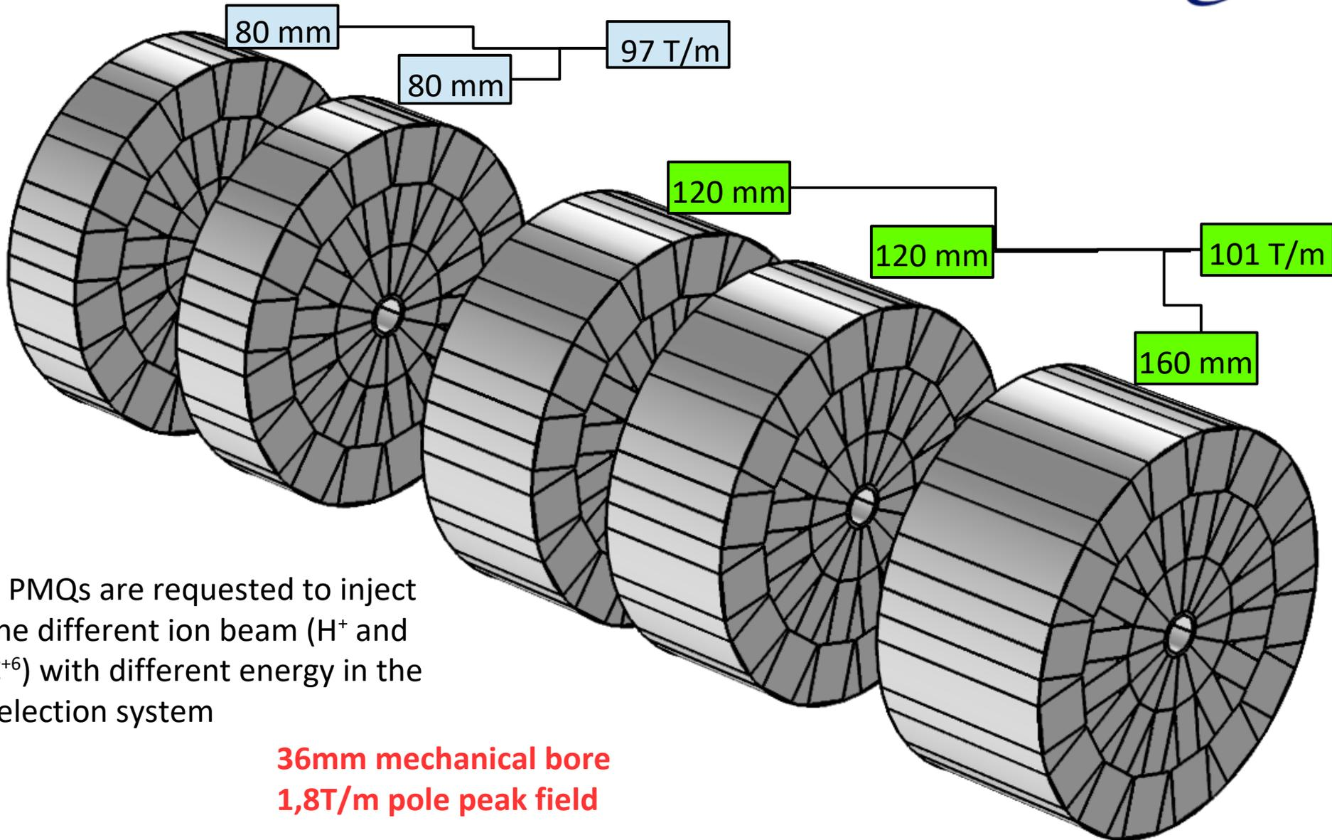
5 PMQs are requested to inject the different ion beam ( $H^+$  and  $C^{+6}$ ) with different energy in the selection system
