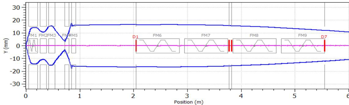
Beam envelope for reference beam 60 MeV protons
