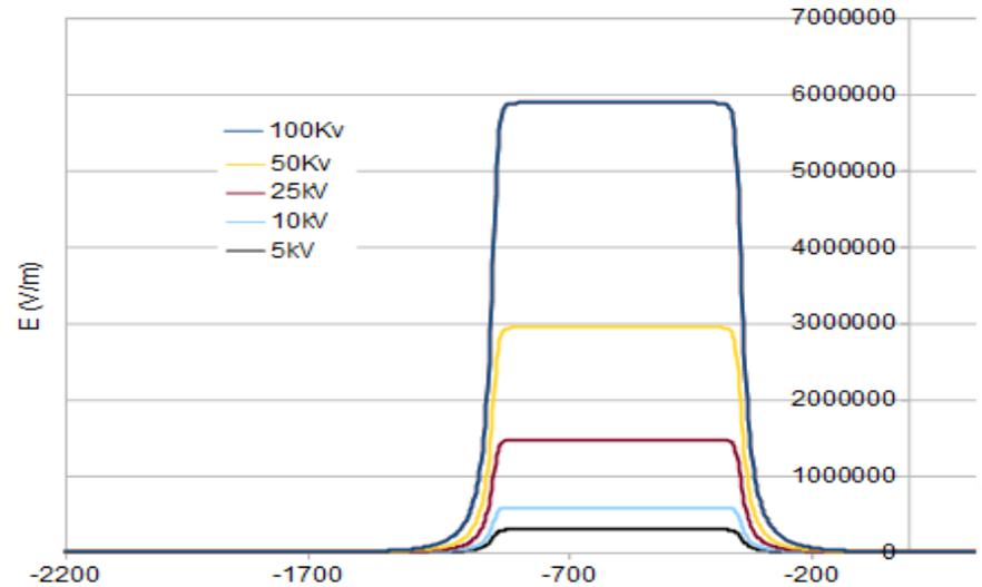
The electric field peak is  $5,88 \times 10^3$  V/mm.
