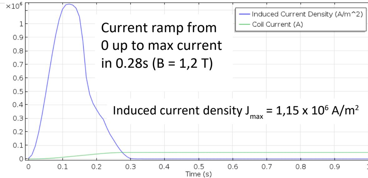
If the current is changed each second (each laser shot) the system could be used as an active energy modulator system
