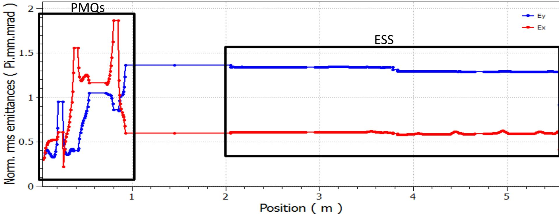
Emittance growth limited to the PMQs system and due to filamentations in the PMQs
