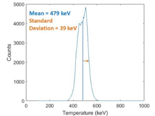
FIG. 5. A histogram of the fitted temperatures from a simple measurement by comparing the predicted output of the diagnostic for different simulated x-ray spectra multiple times. Each time errors from the experimental data are randomly added. The mean is taken as the temperature of the data, and the standard deviation from this mean is the error in the temperature measurement.
