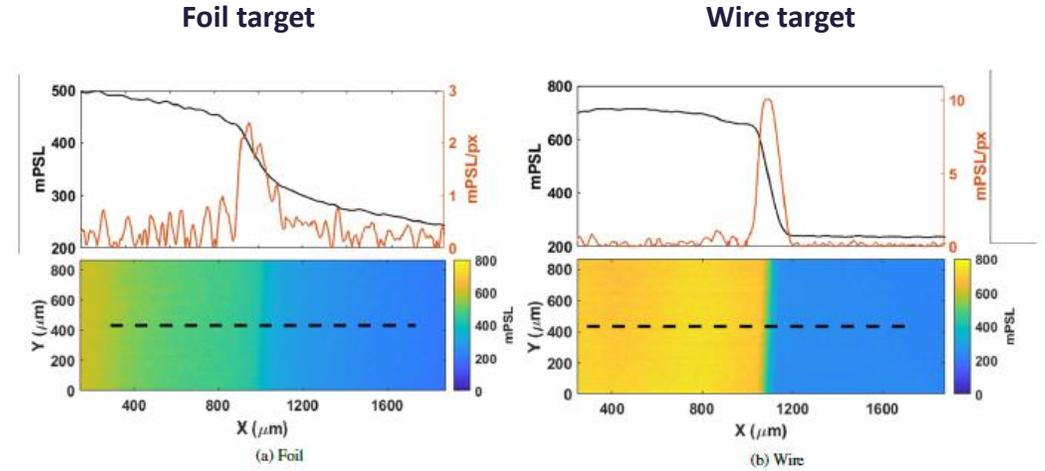
Figure 4: Penumbral radiograph, scale in mPSL (unit of flux for IP), and lineout for a) foil, and b) wire target. The dashed line in each radiograph is where the lineout is determined.
