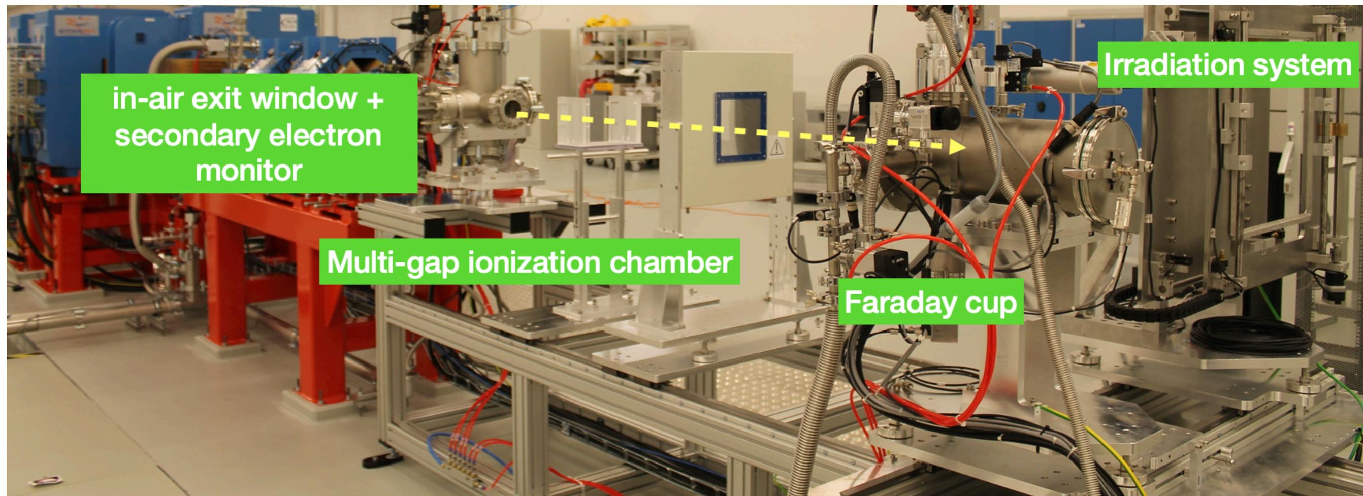
Faraday cup in a special design for absolute dosimetry
