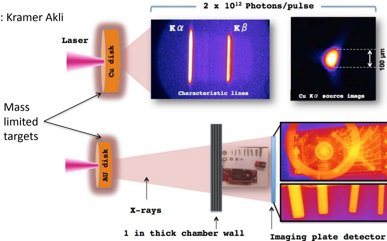
High fluxes and small sources required for high-resolution point projection radiography and Thomson scattering
