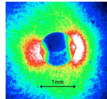
Figure 1 | Snapshot of a flying pellet at the instant of engagement by using a 2ω harmonic laser probe. The probe is perpendicular to the
