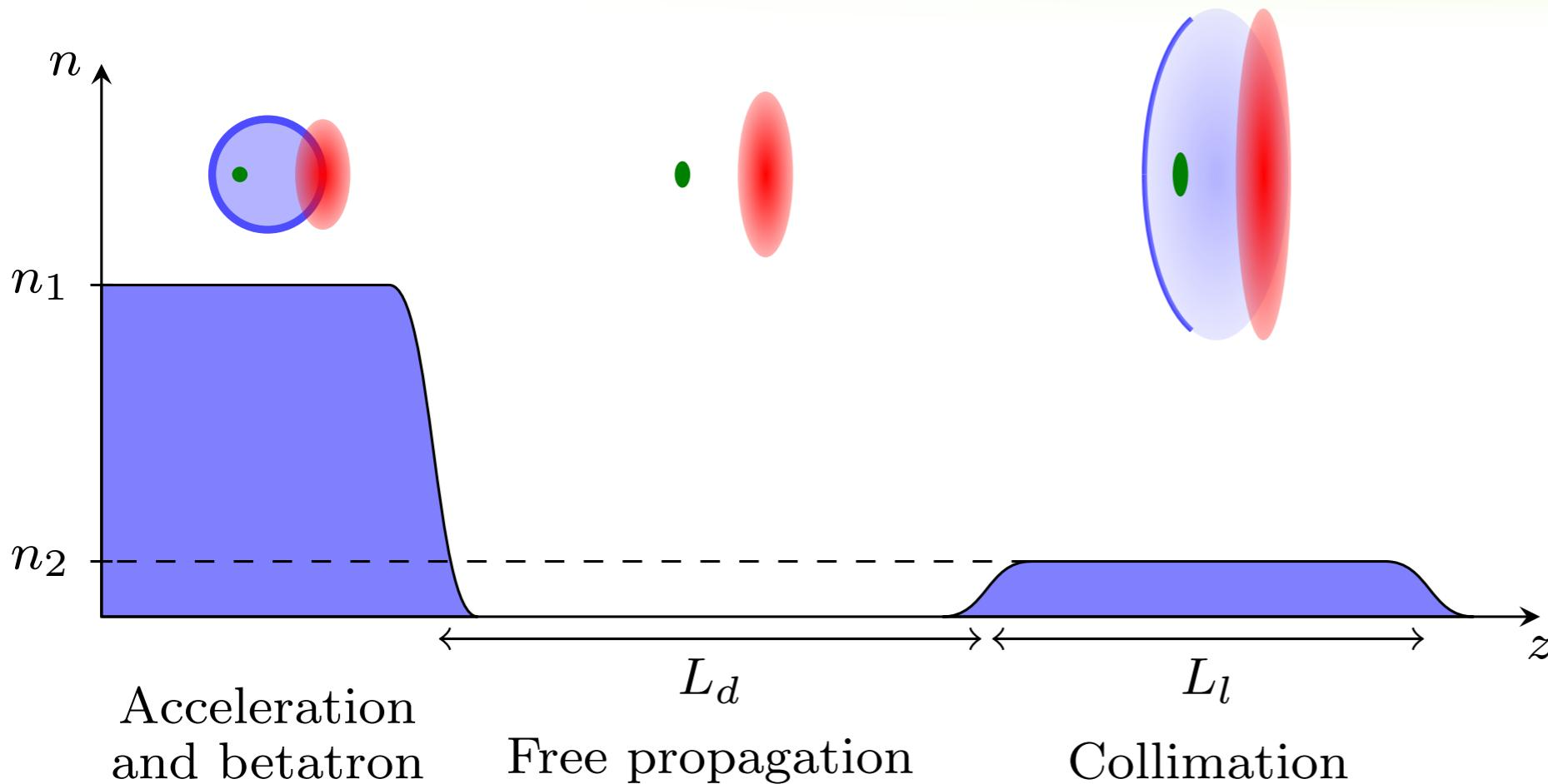
Parameters of the laser-plasma lens :
