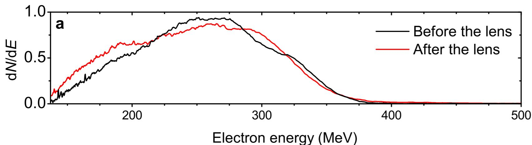
Laser-plasma lens does not disturb the electron energy distribution
