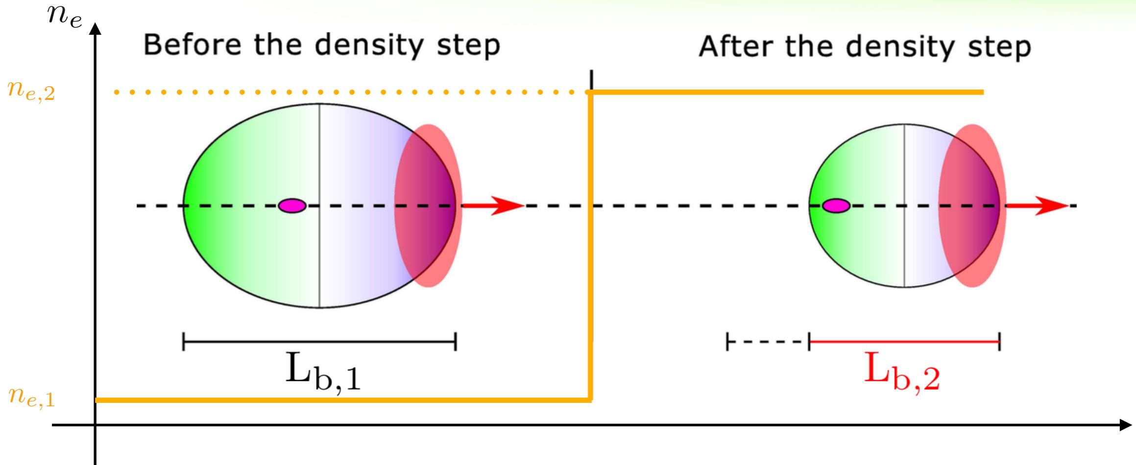
Phase resetting by crossing a sharp upward density transition : the electrons phase slippage is compensated by reducing abruptly the cavity size  $L_b$
