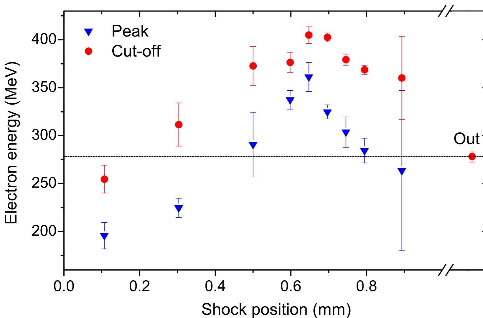
By changing the position of the shock, it is possible to change the energy gain of the peak
