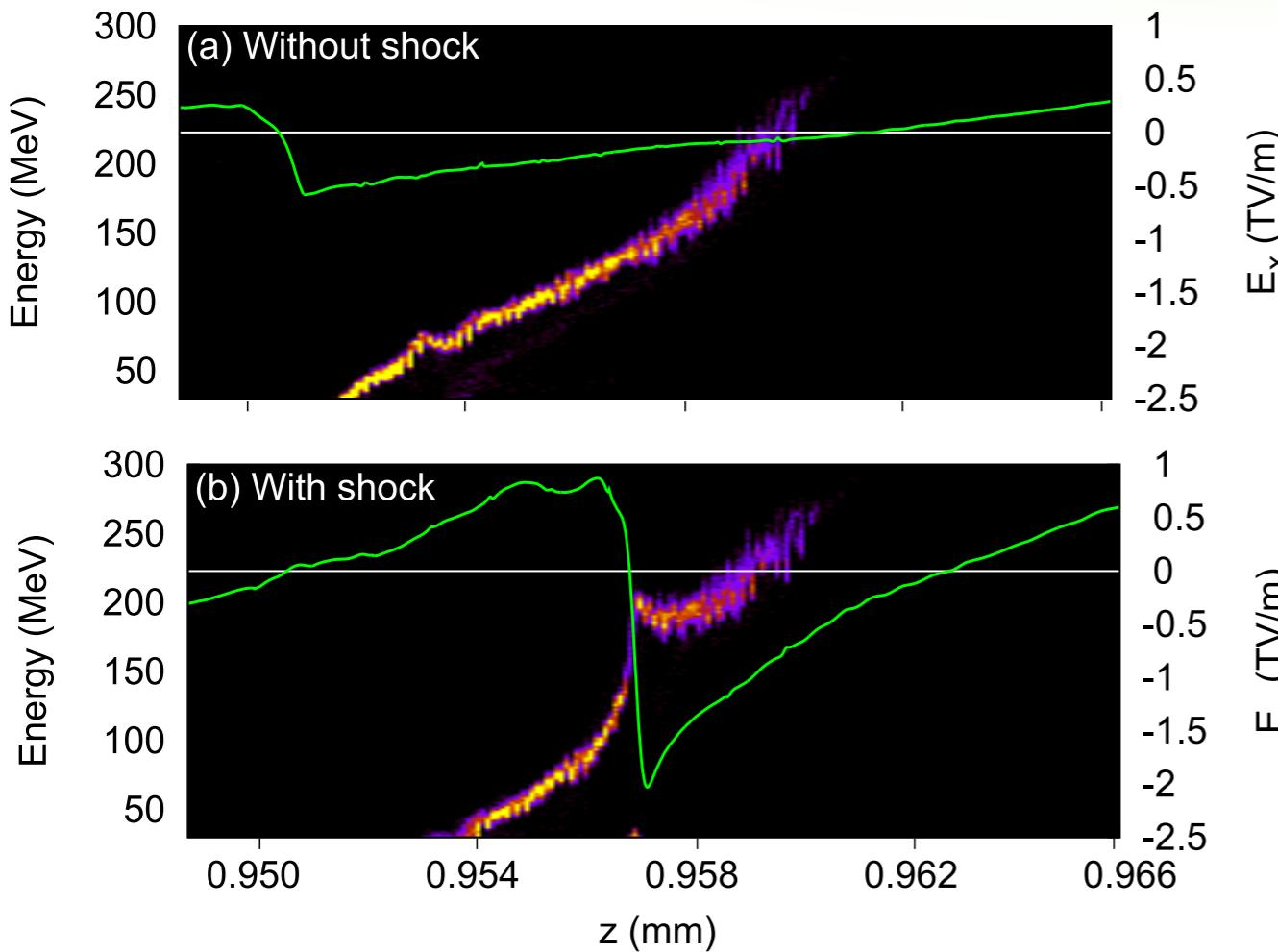
Without shock : lengthly self-injection creates a long electron bunch
