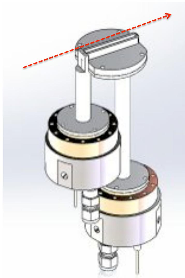
Dual valve assembly – Isometric view
