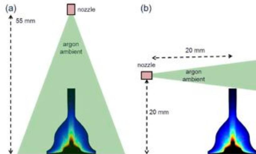
AASC gas nozzle used to inject gas against and across plasma jet
