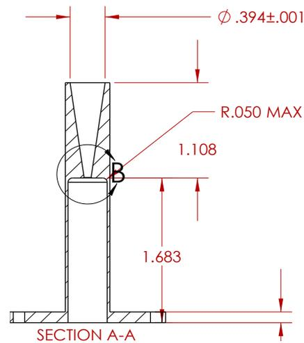
10mm conical nozzle cross-section
