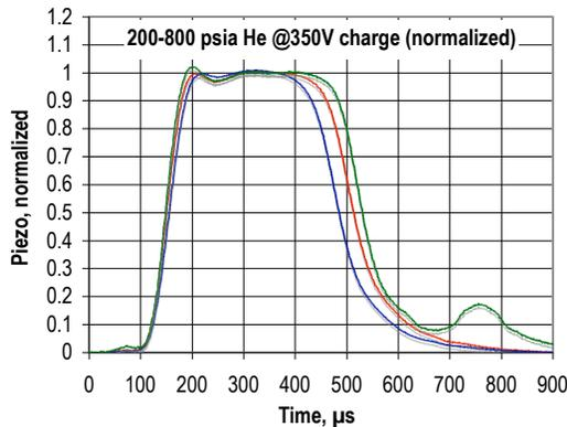
Piezo signals at 350V charge voltage and different pressures
