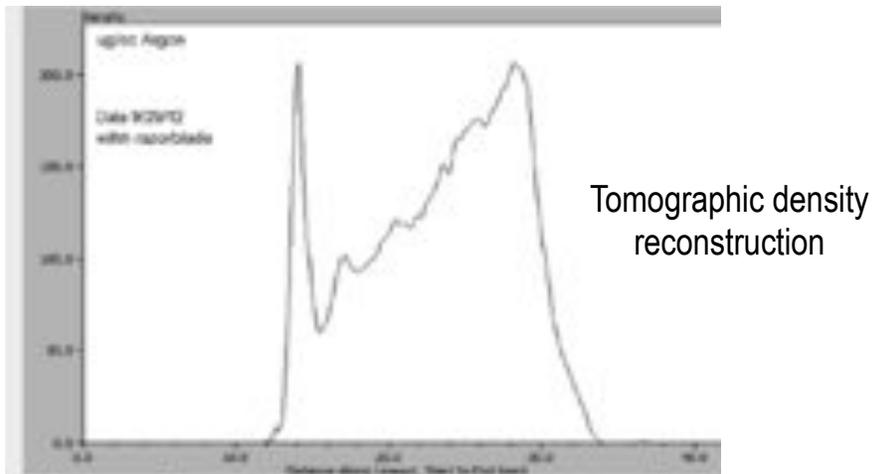
Density profile of a 20mm long region with sharp entrance gradient and linear density ramp (for LPA laser at BELLA)
