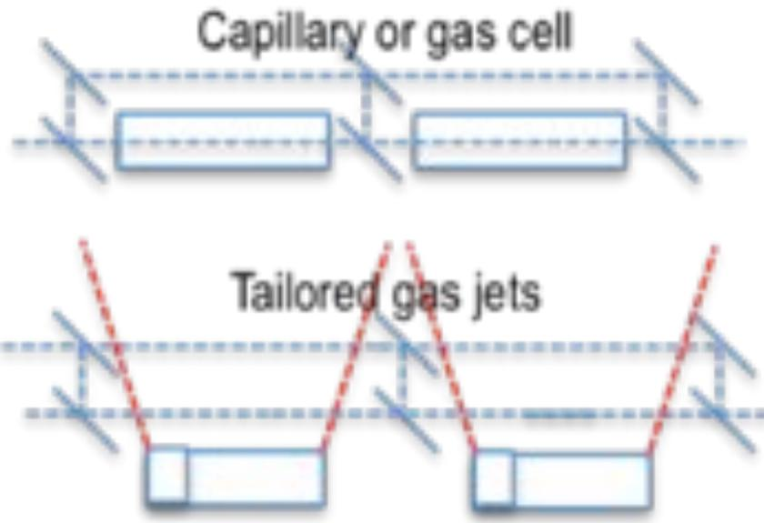
Segmented capillary and gas jet targets for LPAs)
