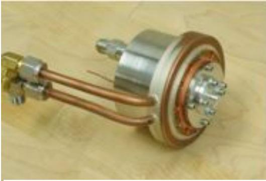
Valve with simple conical nozzle
