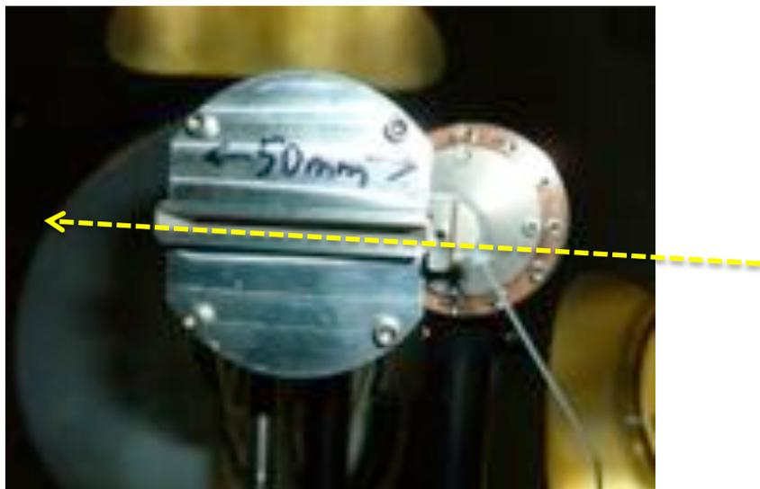
Rectangular nozzle and conical nozzle are driven by separate valves allowing *independent* control of density and gas species, e.g. N<sub>2</sub> doped hydrogen cone, pure hydrogen slit
