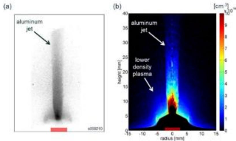
XUV image and simulated image of Al plasma jet produced by 1.4MA/250 ns pulse
