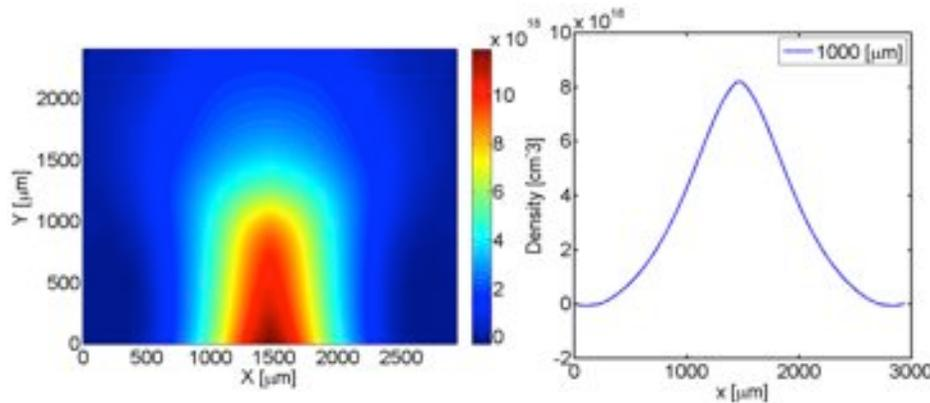
Transverse neutral density profile of He gas jet from 1 mm nozzle
