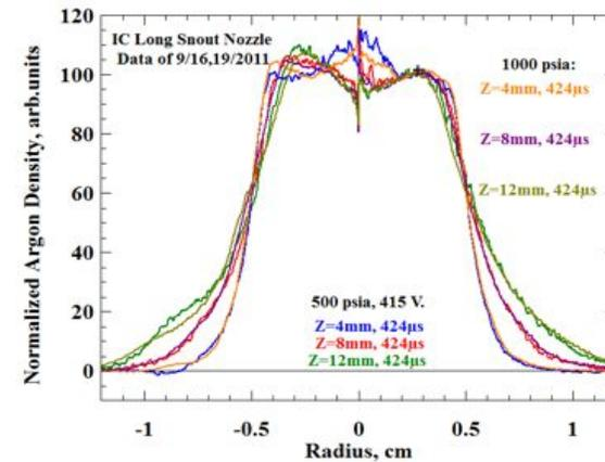
Radial density lineouts (10mm nozzle)
