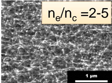
Combination of Carbon-Nano-Tube (CNT) foam with Diamond-like Carbon (DLC) foils
