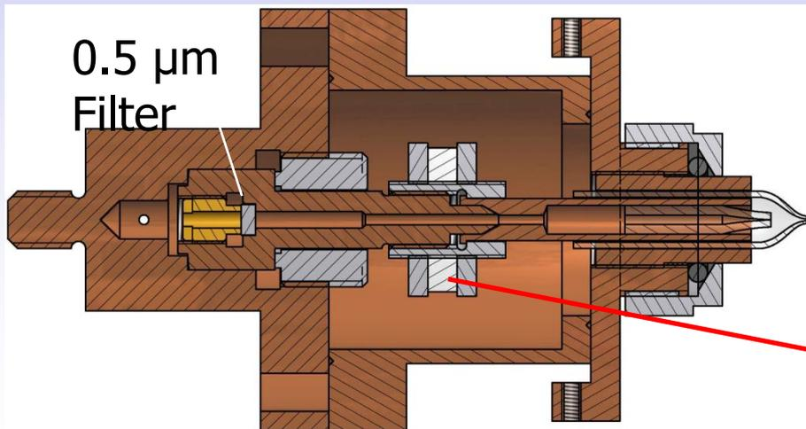
Piezo actuator triggering even breakup of jet to droplets
