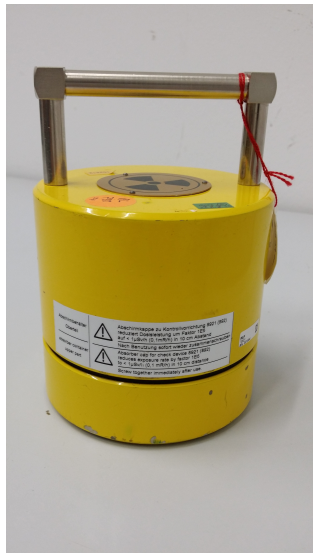
Figure A.4.: Strontium-90-source BL 730 in container mark 8921
