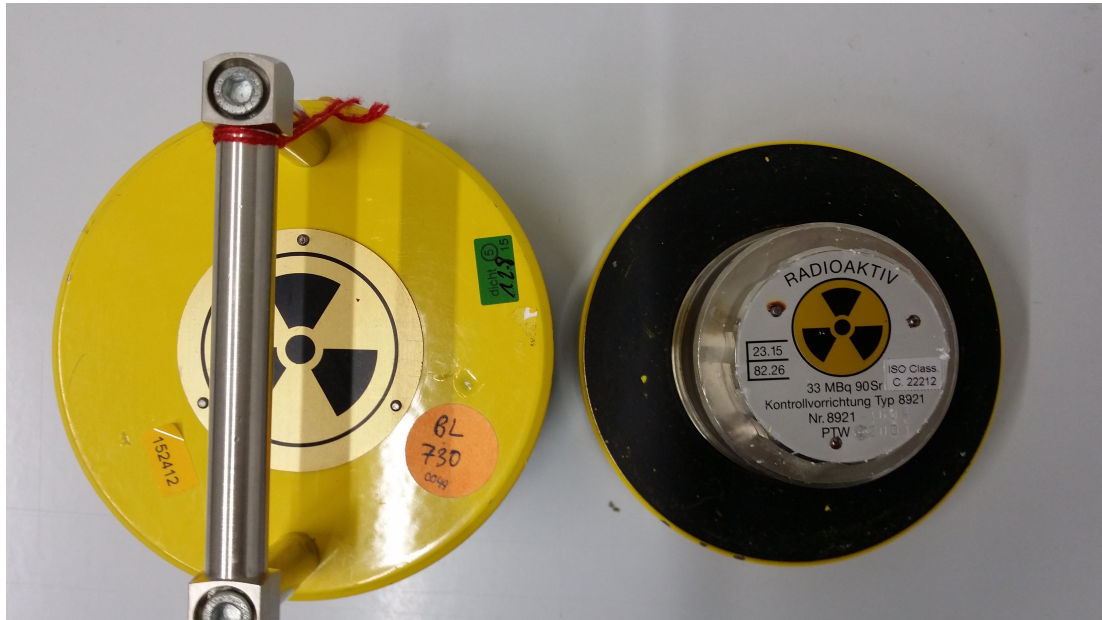
Figure A.4.: Strontium-90-source BL 730 in container mark 8921
